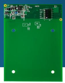
Contactless 13.56MHz ISO/IEC 14443 and NFC ISO/IEC18092, USB-CCID board supports all major PC operating systems and features a power amplifier.
