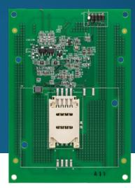
Contactless 13.56 MHz, USB-CCID, ISO/IEC 14443, and NFC module features ISO/IEC 7816 SAM support.
