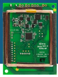
125 kHz and 13.56 MHz mutli-technology smart card reader/writer module features an on board antenna (OBA).
