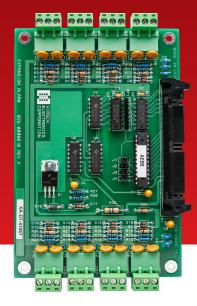
Hirsch's Alarm Expansion Board (AEB8) expands the line module input capacity of a controller. AEB8 provides an additional eight (8) line module inputs per board.
