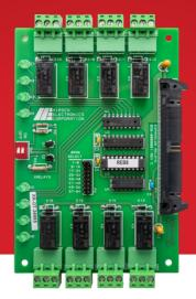
Identiv's Relay Expansion Board (REB8) provides eight (8) additional two (2) AMP form C dry relay outputs, rated for 24VDC. These relays are socketed and removable.
