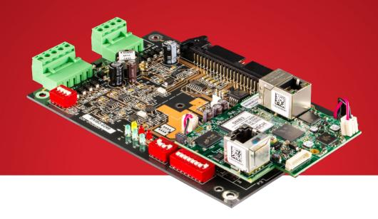
Identiv's Secure Network Interface Board 3 (SNIB3) brings advanced functionality and capabilities to the Hirsch controller line
