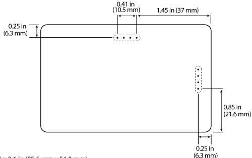
Card size: 3.4 x 2.1 in (85.6 mm x 54.0 mm) Slot hole size: 0.5 x 0.125 in (12.7 x 3.2 mm)
