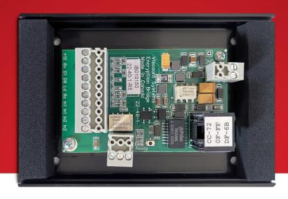
Convert any card reader to a secure IP device, removing the need for conventional control panels.
