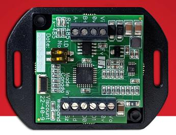
Upgrade Wiegand card readers to RS-485 connectivity, simplifying integration into advanced control systems.
